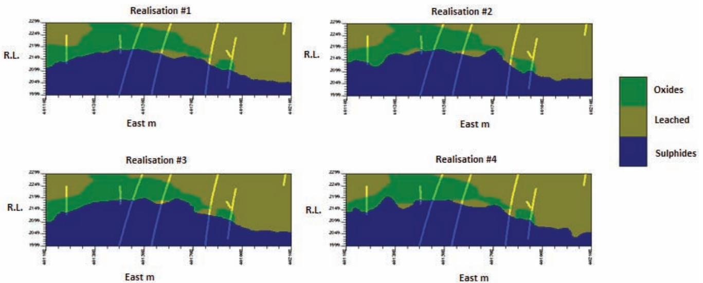
**FIG 5** - East-west profiles of the geological model showing four possible realisations (simulations) of the copper mineral zone model.
