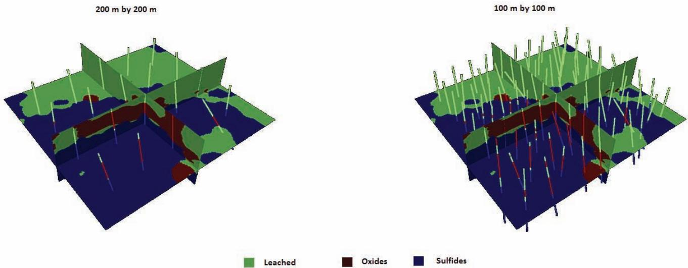
**FIG 7** - Fictitious drill holes spacing and geology simulation of the deposit showing minerals zones models based on drill spacing of 200 m × 200 m and 100 m × 100 m.
