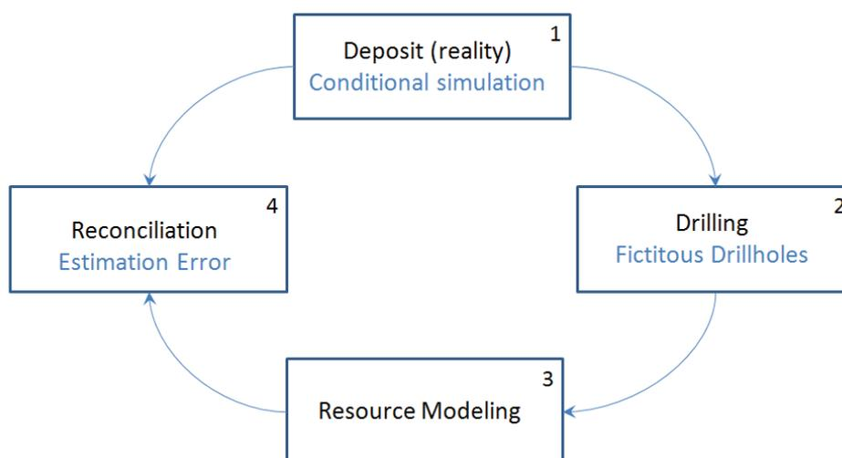
FIG 4 - Workflows of process showing the four main steps to calculate the estimation error for different sampling grid spacing.
