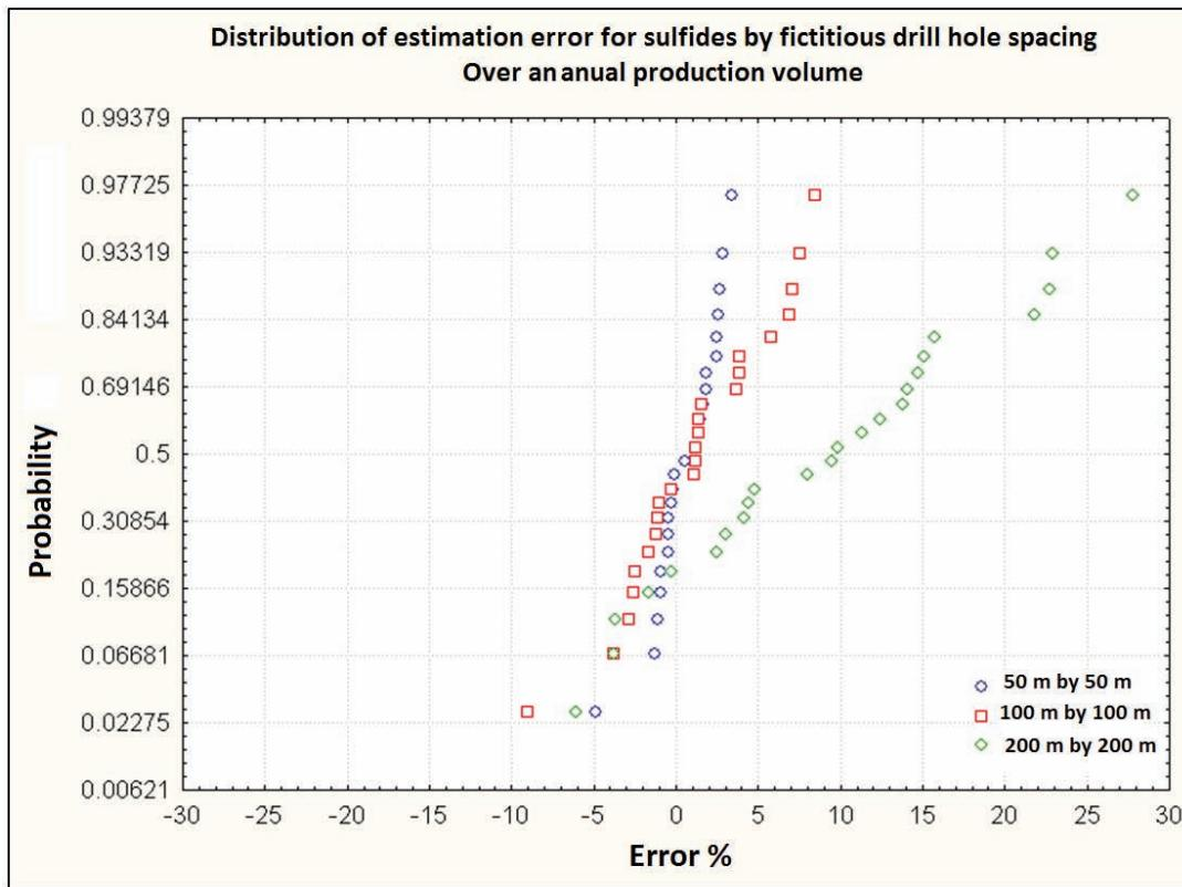
**FIG 11** - Distribution of estimation error for primary ore showing the accuracy and precision of the estimated models based on different fictitious drilling spacing grids.
