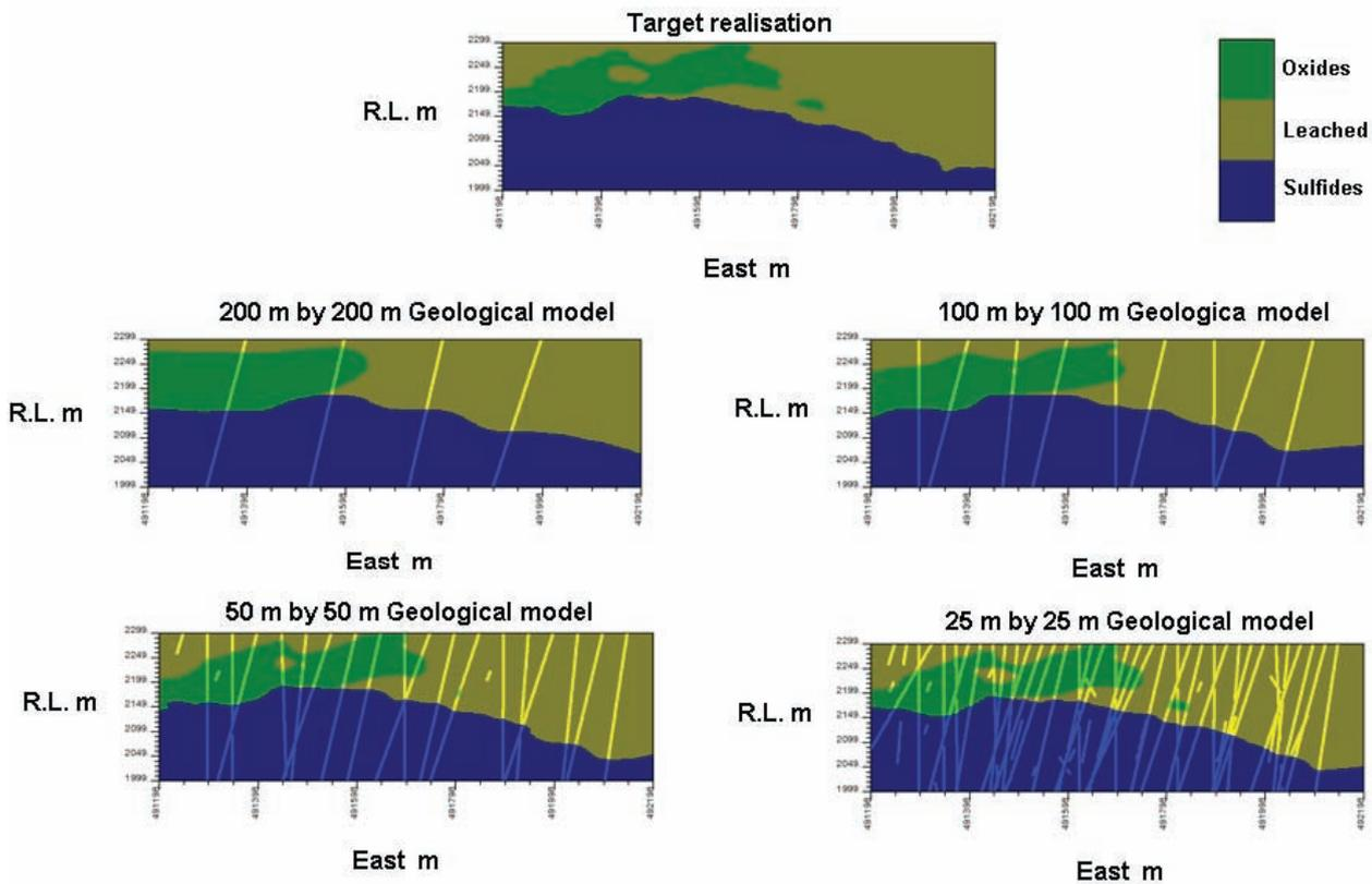
**FIG 8** - Sections of target realisation (unknown reality) versus geological models from fictitious drill holes showing the variations of the geological model respect to different sampling grids.
