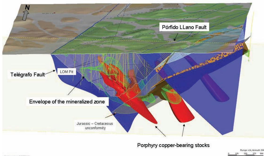
**FIG 2** - Isometric view of the simplified geological model of Telégrafo project showing the relationship between the porphyry and copper (gold) mineralised zones.
