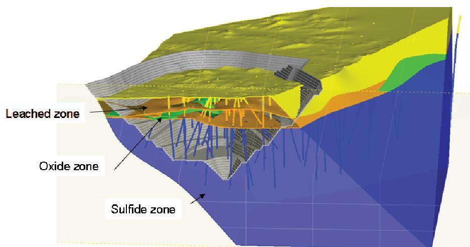
**FIG 3** - Isometric view of the copper mineral zones at Telegrafo project showing the principal geological boundaries. The sulfides zone, the oxide zone and the leached zone.
