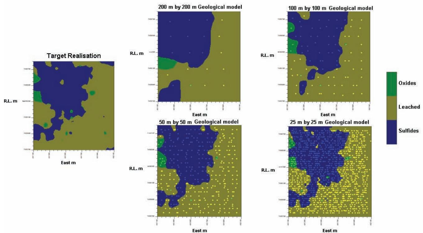
**FIG 9** - Plans of target realisation (unknown reality) versus geological models from fictitious drill holes showing the variations of the geological model respect to different sampling grids.
