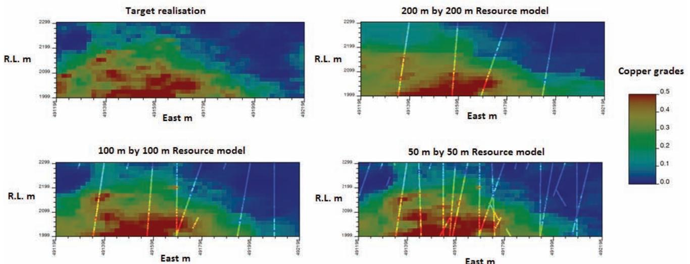
**FIG 10** - Sections of the copper grades target realisation and the estimated copper grade models using fictitious drill holes showing the variations of the copper grades respect to different sampling grids.
