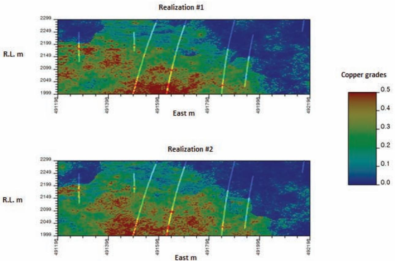
FIG 6 - East-west profile: two realisations of copper grades and conditioning data showing two possible realisations (simulations) of the copper grade.
