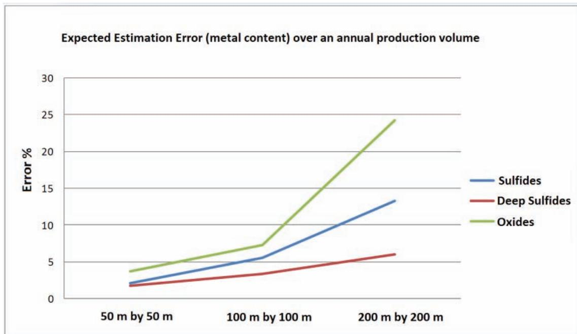
FIG 12 - Expected estimation error (metal content) over annual volume as function of drilling spacing grids showing different behaviour for sulfides ore, deep sulfides ore and oxide ore.
