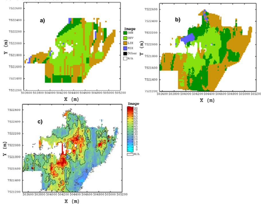
Figure 7: Level 2125 a) deterministic model units, b) probabilistic model units and c) solubility ratio map from cosimulation of CuT and CuS with isocurve.
