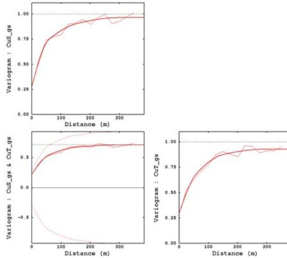
Figure 5: Bivariate experimental and modelled variograms of Gaussian transformation CuS and CuT
