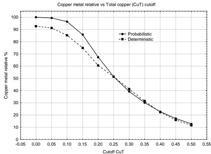
Figure 6: Copper metal relative vs. total copper cutoff of both models
