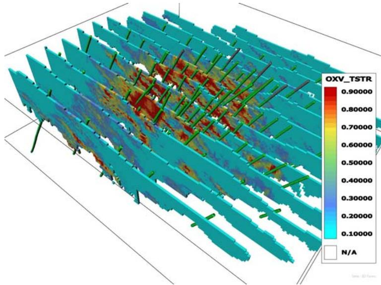
Figure 3: Isometric view, probability or proportions of green oxides and drill hole data
