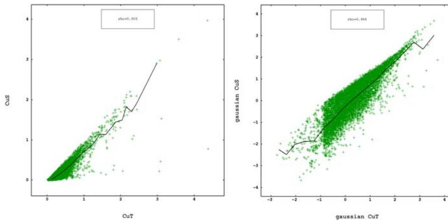
Figure 4: Scatter plot of CuT and CuS on composites 1.5 m with conditional expectation curve (CuS/CuT) on raw data and normal score transformation.
